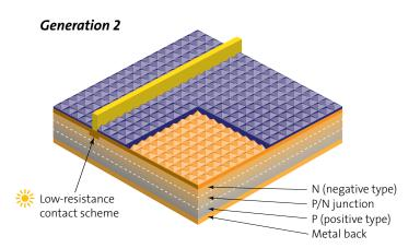
*Localized rear contacts* – By precisely placing rear contacts on the back of the cells, we can further increase our energy conversion by preventing the recombination losses that typically occur at this surface.
